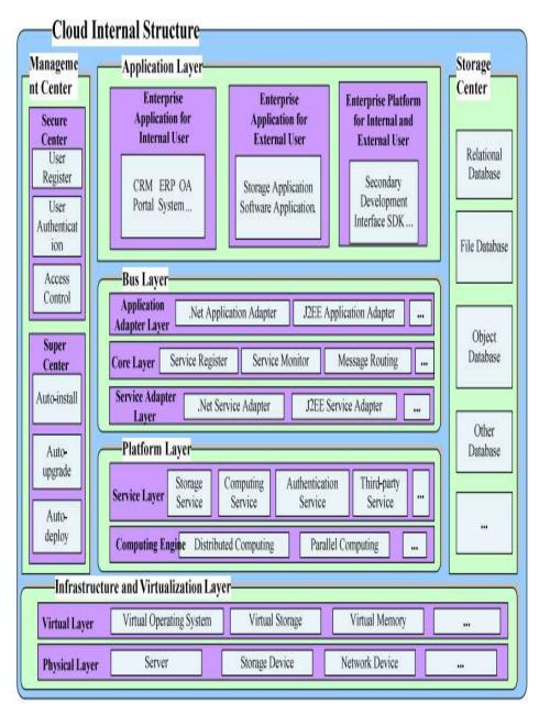
Figure 1.5 Cloud internal structures [20]
