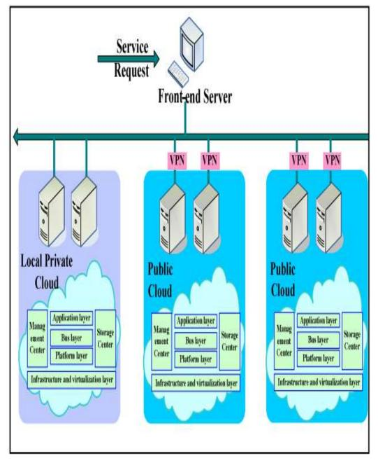
The center of storage is often used for the prices of data processing and it also stores different elements of the cloud environment. Figure 1.4 shows the architecture of hybrid CC.
